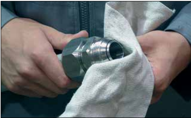
Clean the JIC fittings with a clean cloth.
