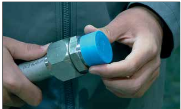
Immediately after flaring and Jetcleaner cover the ends with plastic plugs.
