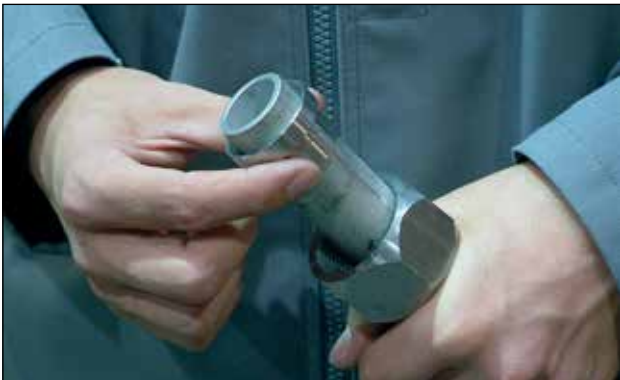
Install nut and sleeve. Measure you have the right outside diameter and wallthickness of tube.
