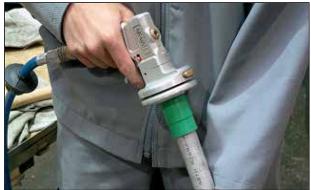
Shoot through two pellets with GS Jetcleaner.
