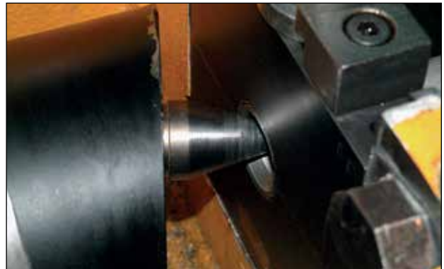
Flare tube end to recommended size (see Table 1 next page). Clean the flaring cone and the end of the tube with a clean cloth. Use oil on the flaring cone and the tube end.
