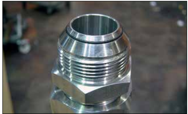
Make sure the O-ring is installed in the recess of the JIC fittings, not damaged or twisted.
